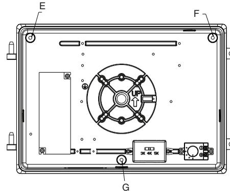
3. Run the main power supply wires through the knockout hole removed in step 2. Connect the main power to the driver according to the wiring diagram.
